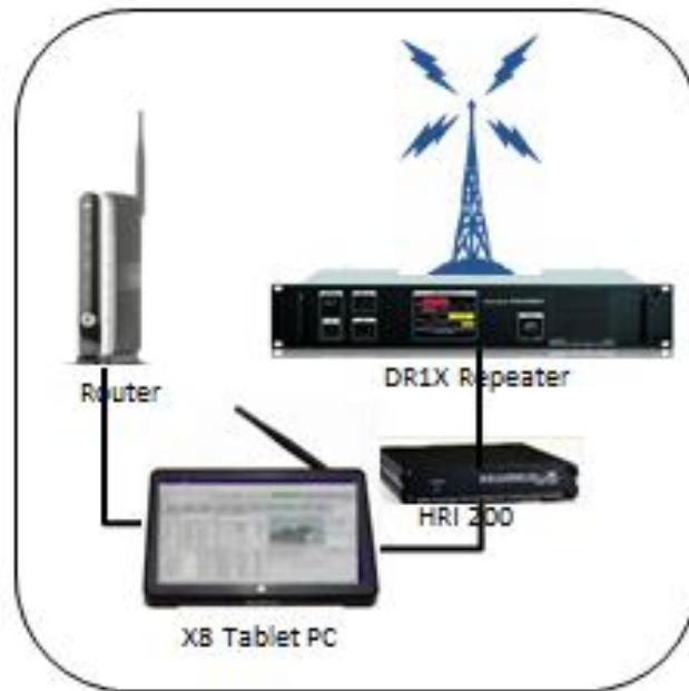
Figure WiRES-X Repeater
