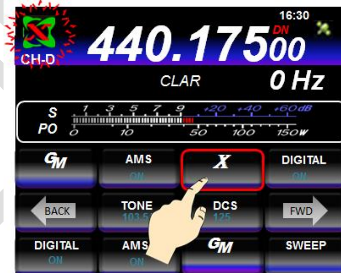
Figure 58 The FT-991 automatically switches to transmit mode and “X” and WiRES-X icon flashes.
