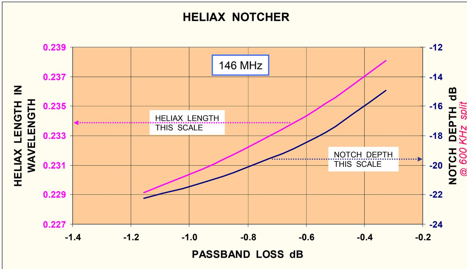
NOTE: Use with a  $\lambda/4$  connecting line. The line adds ~ 5 dB to the notch depth
