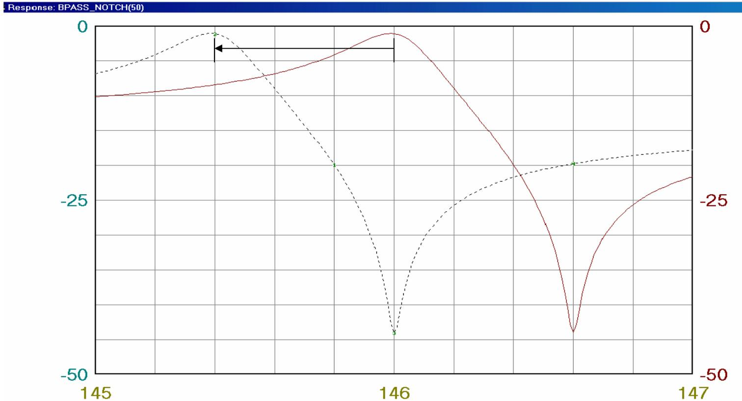
MOVING THE BANDPASS FREQUENCY DOWN MOVES THE NOTCH BY THE SAME AMOUNT 21
