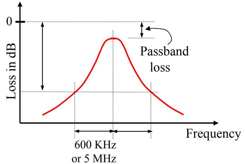
146 MHz Resonator Attenuation at +/- 600 KHz
