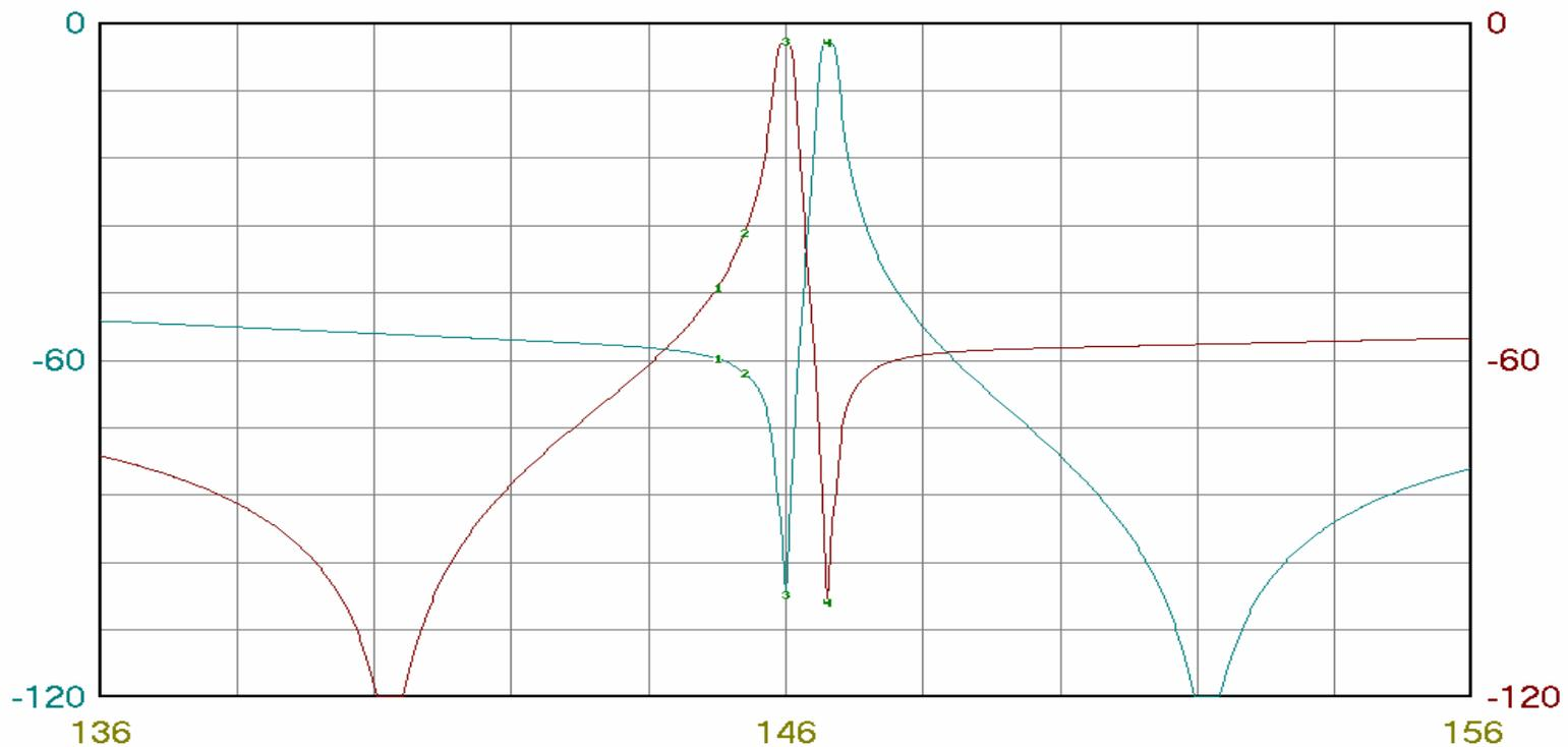
COMPLETE DUPLEXER RESPONSE OVER A 20 MHz FREQ SPAN
