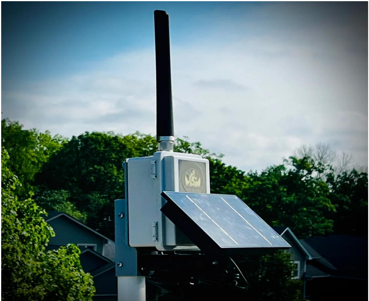
Typical Meshtastic Base station/repeater.
