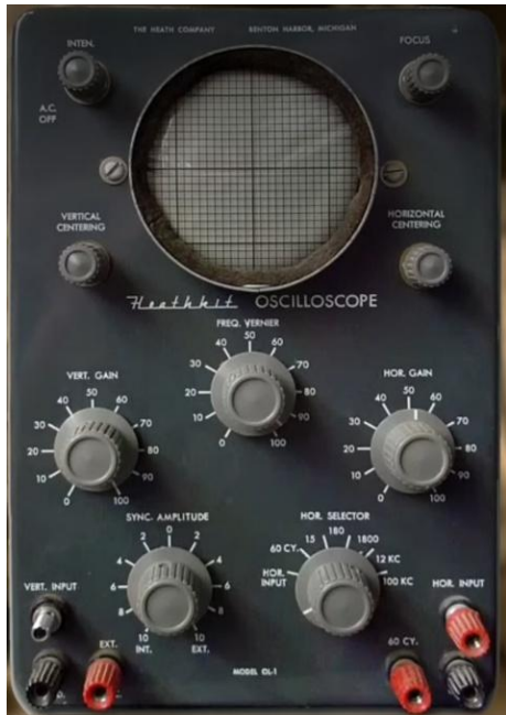
The Heathkit O-1 (or OL-1) classic 5-inch vacuum tube oscilloscope produced by the Heath Company.
