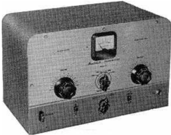
The AT-1, a three-tube CW transmitter introduced in 1955.
