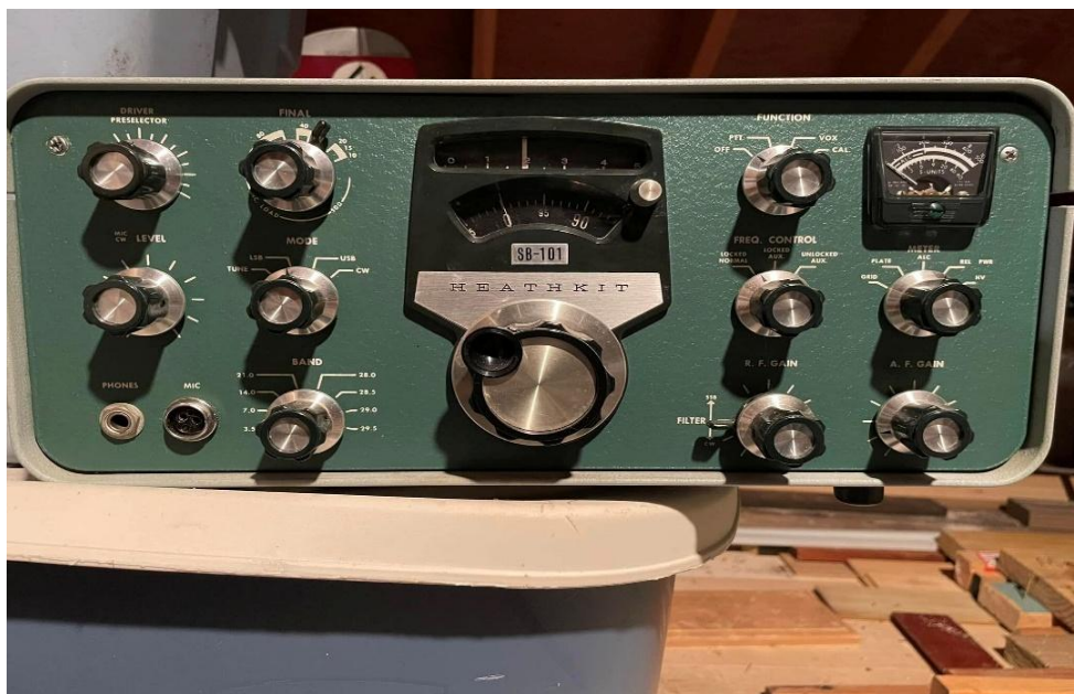
Heathkit SB-101HF SSB transceiver.
