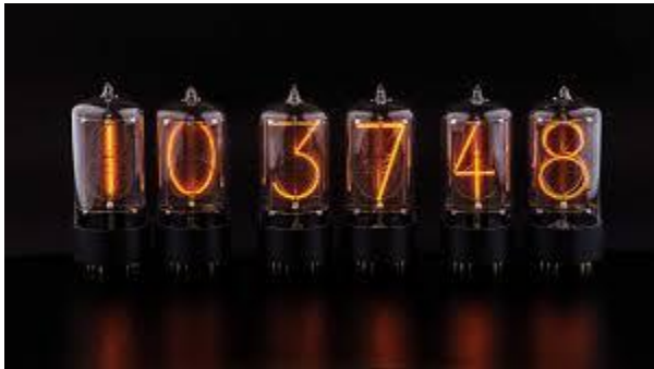
Typical Nixie tube display.
