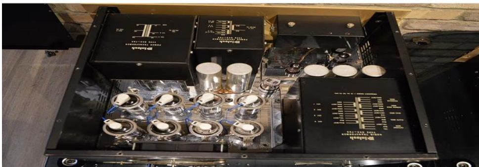
Inside view of a McIntosh model MC – 3500 audio amplifier, similar to what was used on American Submarines during the 1960's & 1970's.
